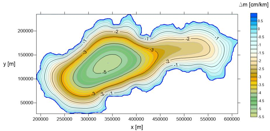
Fig. 11 Differences of the scale distortion values between Lambert's conformal conic projection SR and its modification using LE solved by FEM
