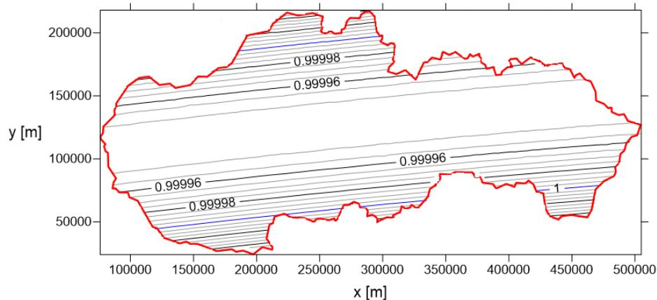
Fig. 6 Isometric lines of the scale distortion factor  $m$  for the Conformal conic projection in an oblique aspect
