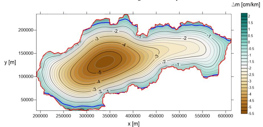
Fig. 12 Differences of the scale distortion values between Conformal conic projection with minimizing RMS in a normal aspect and its modification using LE solved by FEM
