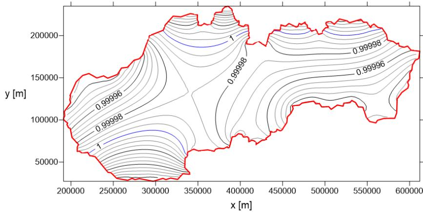
Fig. 2 Isometric lines of the scale distortion factor  $m$  for modification of Lambert's conformal conic projection in a normal aspect using LE solved by FEM
