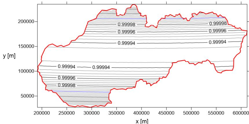
Fig. 1 Isometric lines of the scale distortion factor  $m$  for Lambert's conformal conic projection in a normal aspect
