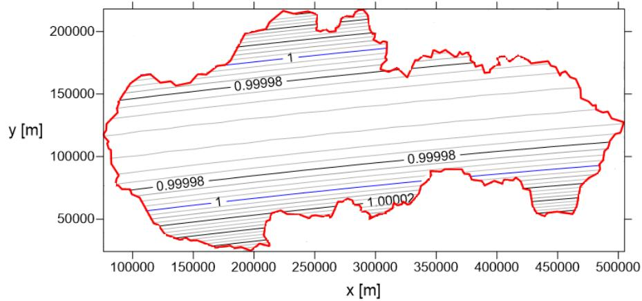
Fig. 8 Isometric lines of the scale distortion factor  $m$  for the Conformal conic projection with minimizing
