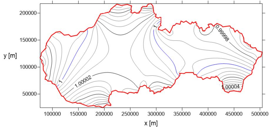
Fig. 9 Isometric lines of the scale distortion factor  $m$  for the Conformal conic projection with minimizing RMS in an oblique aspect using LE solved by FEM
