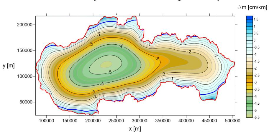
Fig. 13 Differences of the scale distortion values between Conformal conic projection in an oblique aspect and its modification using LE solved by FEM
