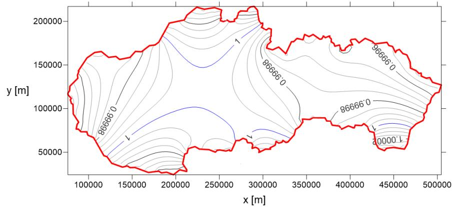
Fig. 7 Isometric lines of the scale distortion factor  $m$  for the Conformal conic projection in an oblique aspect using LE solved by FEM
