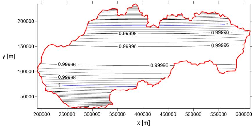
Fig. 3 Isometric lines of the scale distortion factor  $m$  for the Conformal conic projection with minimizing RMS in a normal aspect
