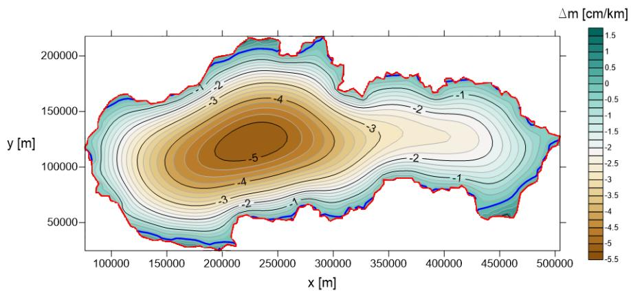
Fig. 14 Differences of the scale distortion values between Conformal conic projection with minimizing RMS in an oblique aspect and its modification using LE solved by FEM
