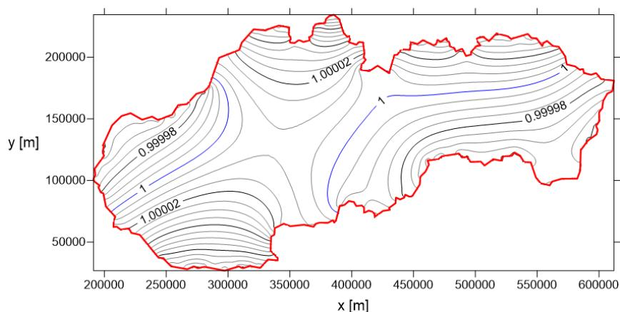
Fig. 4 Isometric lines of the scale distortion factor  $m$  for modification of the Conformal conic projection with minimizing RMS in a normal aspect using LE solved by FEM
